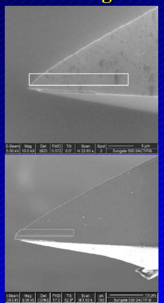
The sample is cut very quickly at the apex of the SACT sample with a taper angle used with the clean-up-cut boxes.
