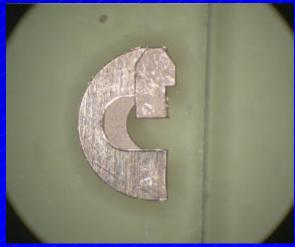
Ready for mounting. Use a dab of epoxy on grid to stabilize it.
