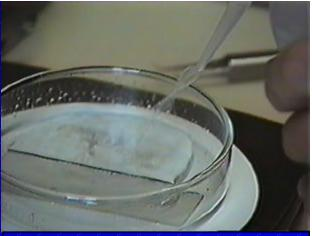
Permanently mount a glass slide in a Petri dish. Fill the dish with distilled water for each new sample. Thoroughly clean dish between uses.
