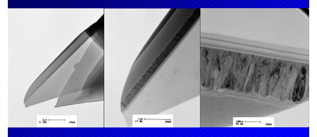
By using a taper, the sample is more robust and less likely to "wave in the breeze." If the substrate is fully removed, then the sample can be cleaned up to remove FIB artifacts in a low angle ion mill.
