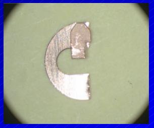
Bend the vertical tab and the handle normally. Use a dab of epoxy on grid when mounting sample to stabilize it.
