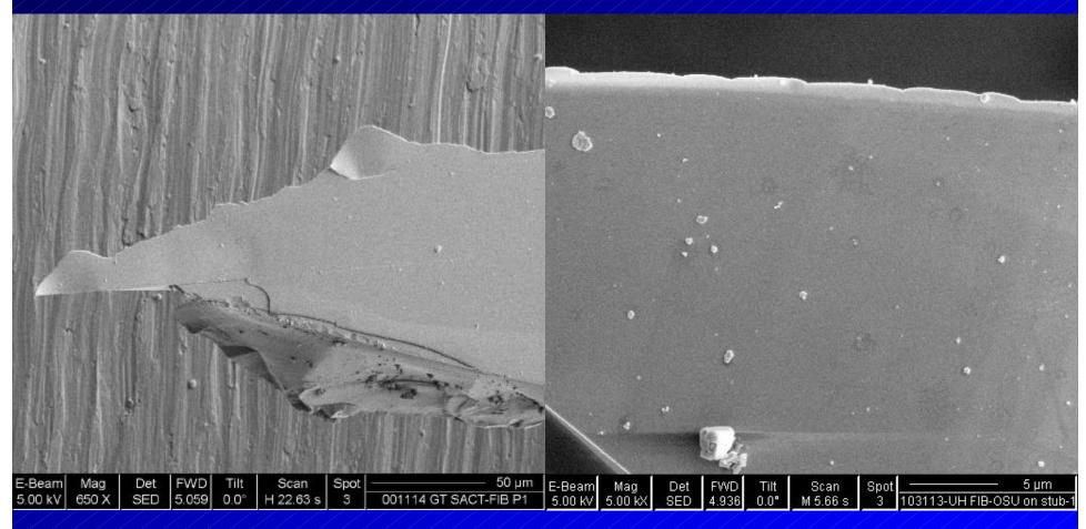
Very thick Nb/Zr multilayer metal coating on Si. The tearing and deformation at edges prevents usable SACT Samples. Samples can be made further back from apex.
