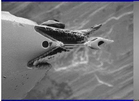
The first test of the SACT/FIB method on a Solarban® 55 coated glass sample showed a crystallite of NaCl at the glass/film interface (arrow). Although cubic holes had been seen in the film, this was the first time that they had been imaged in cross section in the TEM.
