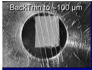
The scribe lines should be relatively deep into the sample, and ideally, they should not be visible from the good side when sample is removed.
