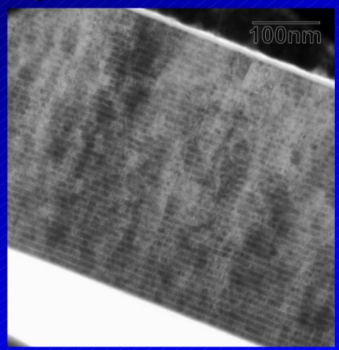
Even with a metallic thin film that has a tendency to delaminate, the SACT/FIB method was able to prepare a sample.
