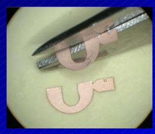
Cut the grids as shown, aligned with tab.
