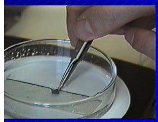
Carefully place sample onto the glass slide with scribe marks facing up. Angle the sample into the water so that it does not float.
